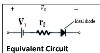
**Equivalent circuit-** Equivalent circuit is a representation of unknown device in the form of known circuit elements like resistor, voltage source etc. This representation presents approximate behaviour of diode on the basis of piece-wise linear characteristics. From piece-wise linear characteristics we can see
