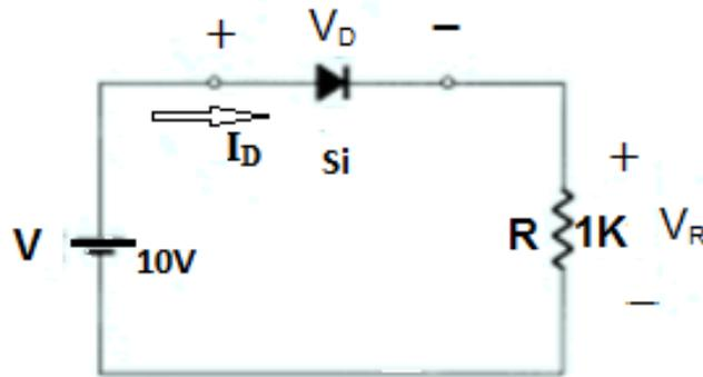
Find  $I_D$ ,  $V_D$  and  $V_R$  in above circuit using equivalent circuit of diode with approximations.
