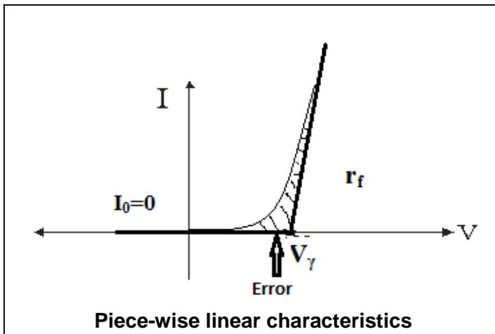
From above discussion it is clear that for actual on paper analysis of diode we have to use nonlinear graph in graphical analysis and exponential function for mathematical analysis. Nonlinear exponential functions are tough to analyse. To simplify our analysis we compromise with some error and use approximate characteristics of diode. In this approximate characteristic we assume that diode shows zero current for all
